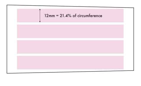
= PRINTING SECTION (21.4% OF THE CIRCUMFERENCE) \*\*\* Max printing sections per set up is 4 \*\*\* Artwork will determine if we can increase to 22% or dial back to 20% to avoid stretching
